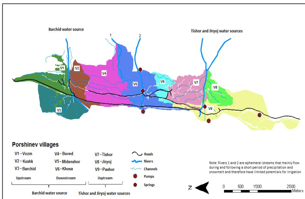
**Figure 2: Water sources and irrigation infrastructure in Porshinev, GBAO, Tajikistan.**
